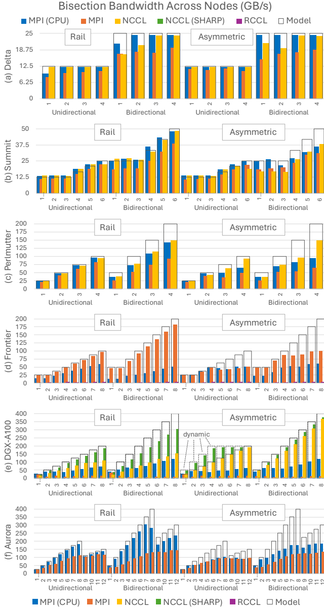
Figure 10: Bisection bandwidth profiles across two nodes were measured with blue (CPU-Only MPI), orange (GPU-Aware MPI), yellow (NCCL), and purple (RCCL) bars. Hollow bars show the proposed model in Equations (1)–(2). Group-to-group patterns gradually change the workload across nodes to expose hardware differences across systems, testing libraries’ performance portability and helping developers make choices for moving their applications across systems.
